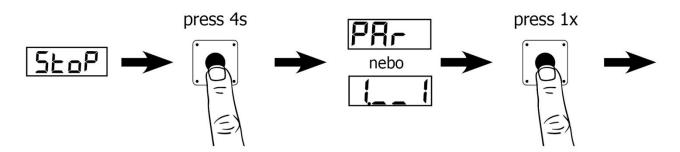
Description of setting of optional parameters on display device. To enter the setup we have to hold knob button and after 4 seconds display shows "Par" ", Par" /or  $1_1 1 0$  — direct display of parameter No.1 — valid for versions supplied until 04/2015.
