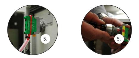
Do not connect any external controls or any other devices before setting the end switches — it can cause automatic start, which is not restricted due to the unset end switches.
