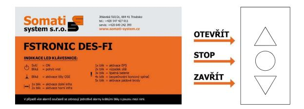
On control panel of FSTronic there is installed keyboard with buttons OPEN, STOP, CLOSE. On the keyboard there are also LED diodes, which display all current states of the control. This enables the gate operator to determine particular states and potential gate alarms
