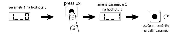
After displaying "Par" press knob button to display individual parameters and their set value.
