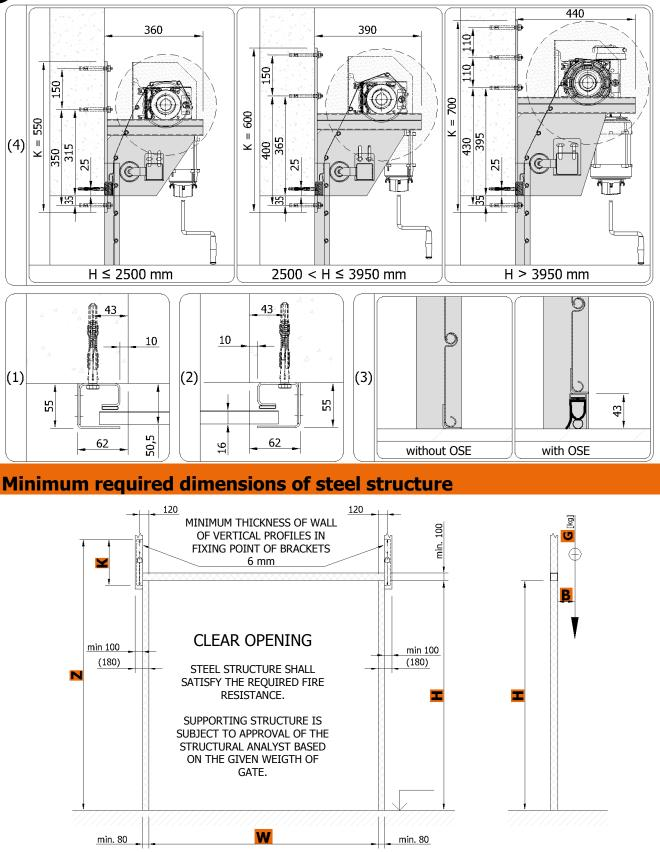
Construction readiness of the opening is secured by the customer according to the requirements of the contractor and depending on the type of jamb and lintel of the opening.
