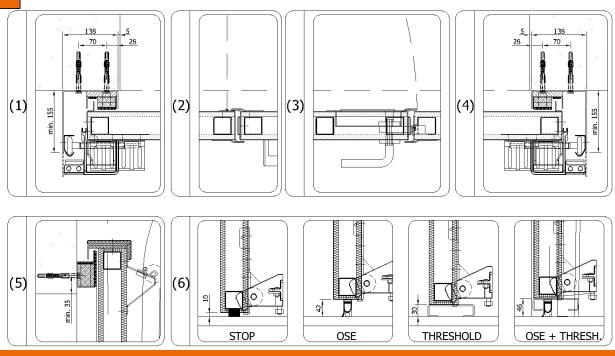
**Minimum required dimensions of steel structure**
