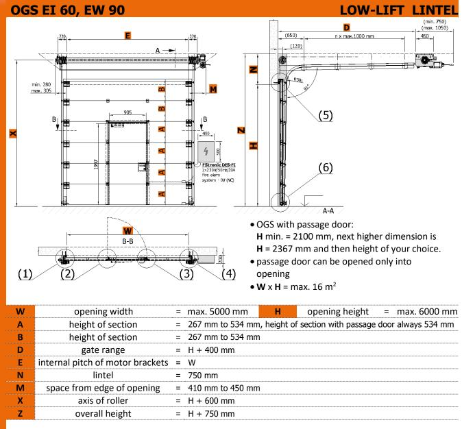
Average weight of gate leaf = 70 kg/m<sup>2</sup> (EI 60) Average weight of gate leaf = 55 kg/m<sup>2</sup> (EI 15 to EI 45, EW 15 to EW 90)
